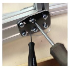
If any nut fails to catch hold it with a small screwdriver or allen key. (If it falls off completely you will need to start over with that piece- be sure to back off the screw tension such that the slack is inside, where you need it, not outside.)
