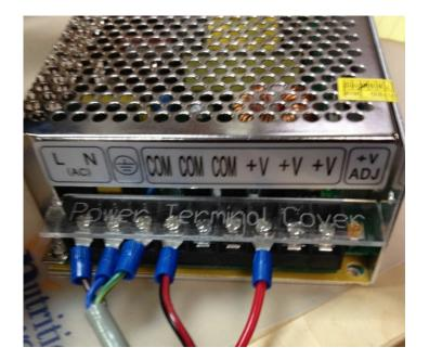
any V+ point (all are equivalent.) Attach the power cord connections as follows: brown to live (L), blue to Neutral (N) and green to ground (see image.) In this case the "black" wire still had some red insulation on it. Be careful that you are using the right wires.
