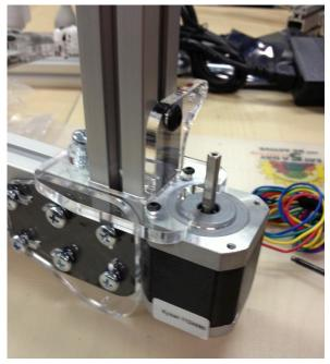
Attach the horizontal portion to the bottom track with a screw, then a washer, and then the and acrylic spacer on the inside of the Z bar.
