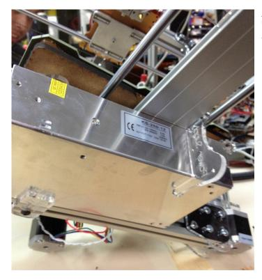
Attach the power supply to the machine; be sure it is solidly attached. This is the view from below the machine.
