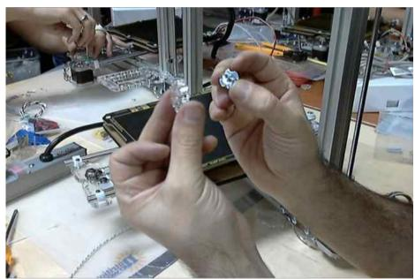
Put a spring in between the heated platform and the wood board. Run the screw though and put the flower adjuster ends on the bottom. Tighten all around. Fully compress the springs for now (you will back these off to align the platform later.) Set the glass piece aside- you will put that on top at the very end of the process.
