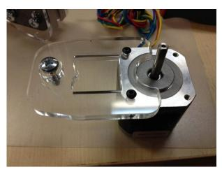
Attach a motor motor to each one as shown (this is the right-hand motor). Then slide them down the Z (vertical) rails on each side with the motors on the outside. They will slide down the Z (vertical) rails on each side. The wires should be in the "back" of the Bukobot. The longer part of the Y carriage is the front, and "right" means "right from the perspective of someone at the front."
