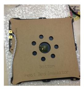
Pick up the heated platform assembly and piece of cardboard. The cardboard is an insulator to make the platform more efficient in holding temperature.
