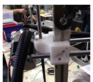
Next assemble the X end stop just like the y one. It will go into two small holes in the left-side (motor side) X end. These holes are hard to see; this picture has highlighted them with a marker and
