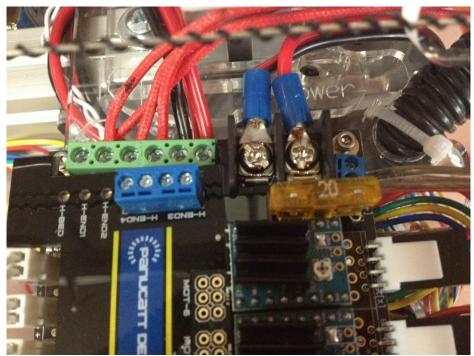
Strip the ends of the extruder heater wires and insert them into the "H-end" pairs on the Azteeg board (if you only have one extruder, just use #1). Since these wires are not quite long enough to go down and through the connector board mount, you should separate them out a bit higher than the end of the cable conduit and run them across the TOP of the connector board
