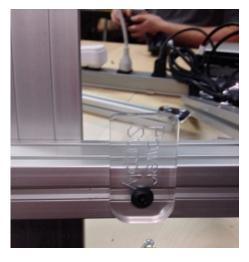
Drop a nut into the track on the very bottom of the Bukobot and attach the smaller "power supply" tab on the left side, sticking out forward. It is a little fiddly to get the nut in (you will have to wiggle it around to get it into the slot and flat). It is also a little hard to get it to catchyou may need to hold the nut in the track with another screwdriver again. You will adjust this significantly at the very end of the build- we are just putting it in a safe place for now.
