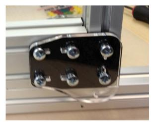
Then, attach ONLY the FIRST side beam. You can use what will be the top as a stop to guide how far down to push it. The bottom of the center aluminum rails should be flush with the bottom of the side rails.
